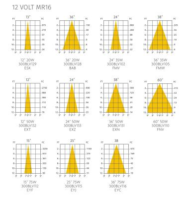
A Aiming angle of fixture, measured from 0° DH Vertical distance from fixture to
