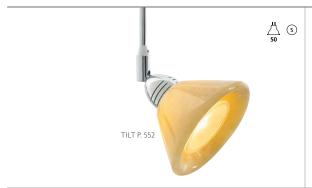
Natural onyx cone. Includes optional Snap Louver Lens Holder. Can hold one lens or louver. Low-voltage MR16 lamp of up to 50 watts. Available for use on Aero, Helios\*, Roto, Tilt, Torpedo Pendant (sold separately).
