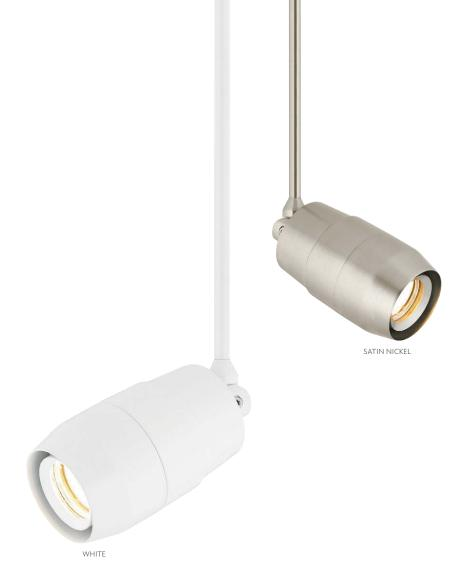
Die cast aluminum LED head, pivots vertically 90°, rotates horizontally 360°. Features horizontal locking mechanisms. Front air intake design allows airflow past internal heat sink fins to rear exit vents while conserving a clean, thoughtful and seamless form. Three interchangeable optics: 15°, 25° and 40°. Holds up to two PAR16 / MR16 lenses or louvers, sold separately.
