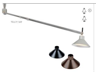
Decorative metal shade. Includes Snap Louver Lens Holder. Can hold a single lens or louver. Silver and black for MR16 of up to 50 watts. Antique bronze for MR16 up to 20 watts only. Available for use on DJ-Archie, DJ-Telescope, DJ-Wally Lite, Joshua Ceiling, K-Pivot, K-Telescope, MO-Pivot, Tele, Wall Telescope (sold separately).
