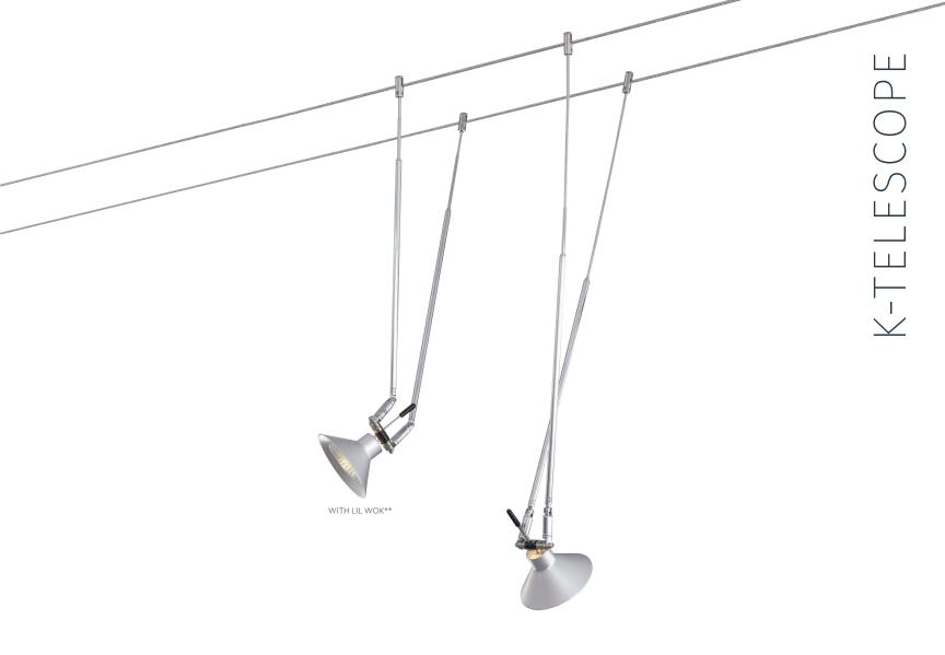
Arms telescope individually from 12-42", creating unlimited angles. For cable separations of 1" to 48". Head rotates 330° and has swivel and pivot action to direct the beam.
