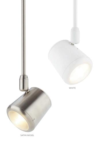
A simple, tool-free, one-handed turn of the outer ring continuously adjusts beam spread from 20° to 50° to avoid the restriction of factory-set optics. Additionally, a locking mechanism with indicator markings ensures precision adjustment of multiple fixtures allowing consistency of fixtures throughout an environment.
