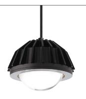
A precision die cast aluminum body serves a dual role as a geometrically striking design detail and the heat sink for this line voltage LED pendant. An optical grade pressed glass lens effectively distributes the output for excellent task lighting on the surface below while eliminating horizontal glare.
