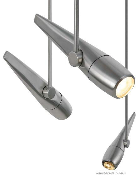
Inspired by advanced aerodynamics, this sleek LED head features a die-cast aluminum tail which also serves as its heat sink. The head rotates 360°, pivots 210° and is available in two beam spreads, 25° or 40°.
