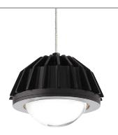
A precision die cast aluminum body serves a dual role as a geometrically striking design detail and the heat sink for this low voltage LED pendant. An optical grade pressed glass lens effectively distributes the output for excellent task lighting on the surface below while eliminating horizontal glare.
