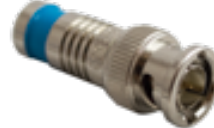
SCP Part No.: 925-6Q-N BNC Compression Connector for RG6/U Quad Shield, Nickel Plated with 6 color bands Packaging: 10 Ea/Bag Package Wt: 0.36 lbs / 0.16 kgs
